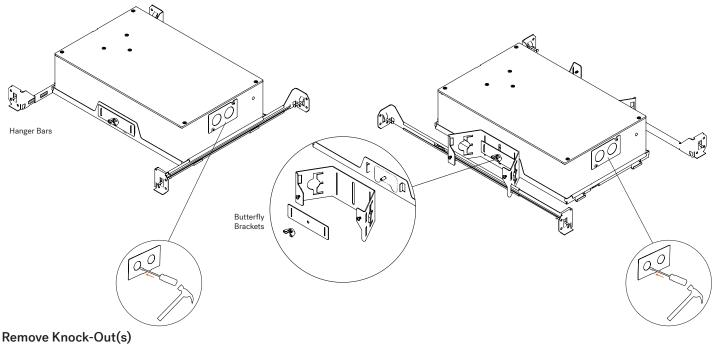
Remove knock-out(s) where needed with a flat-head screwdriver and hammer.
