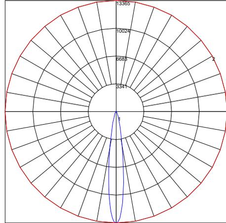
Maximum Candela = 13365 Located At Horizontal Angle = 0, Vertical Angle = 0
