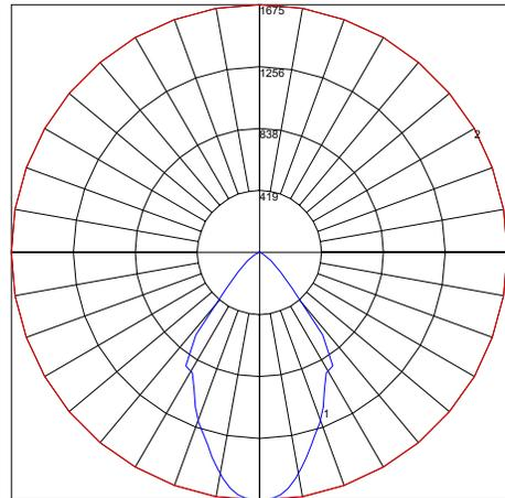
Maximum Candela = 1675 Located At Horizontal Angle = 0, Vertical Angle = 0
