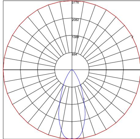
Maximum Candela = 2776 Located At Horizontal Angle = 0, Vertical Angle = 3
