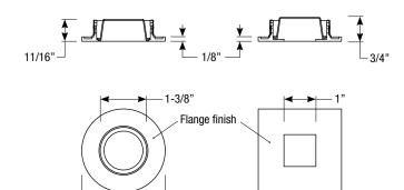
Note: Open reflector does not allow adjustable mechanism to tilt
