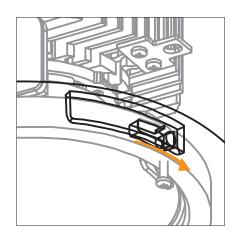
B. Twist module to lock in place
