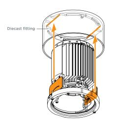
A. Install module into diecast fitting
