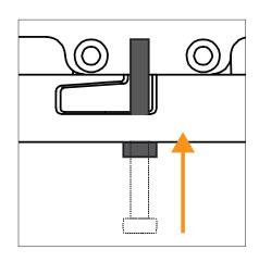
C. Screw module into diecast
