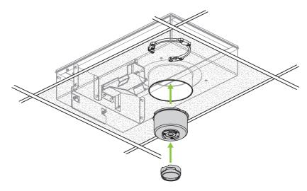
Step 2-1 : Aline the module with the twist lock bracket.
