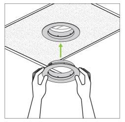
Step 3-2 : Push up the reflector into the flange.
