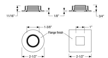
Note: Baffle downlight does not allow adjustable mechanism to tilt
